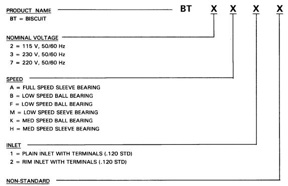
X = E/M VARIATIONS / FEATURES, INCLUDING MOUNTING, TERMINATION (HARNESS), LEAD LENGTH, ETC., NOT AFFECTING BASIC FAN PERFORMANCE.
