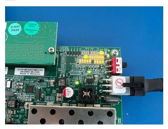
For the System Controller, the DS42 SYSCTRL Init LED comes on immediately and the DS44 SSYCTRL Done LED comes on a fraction of a second later. DS43 SYSCTRL status never lights up - does it do anything?
