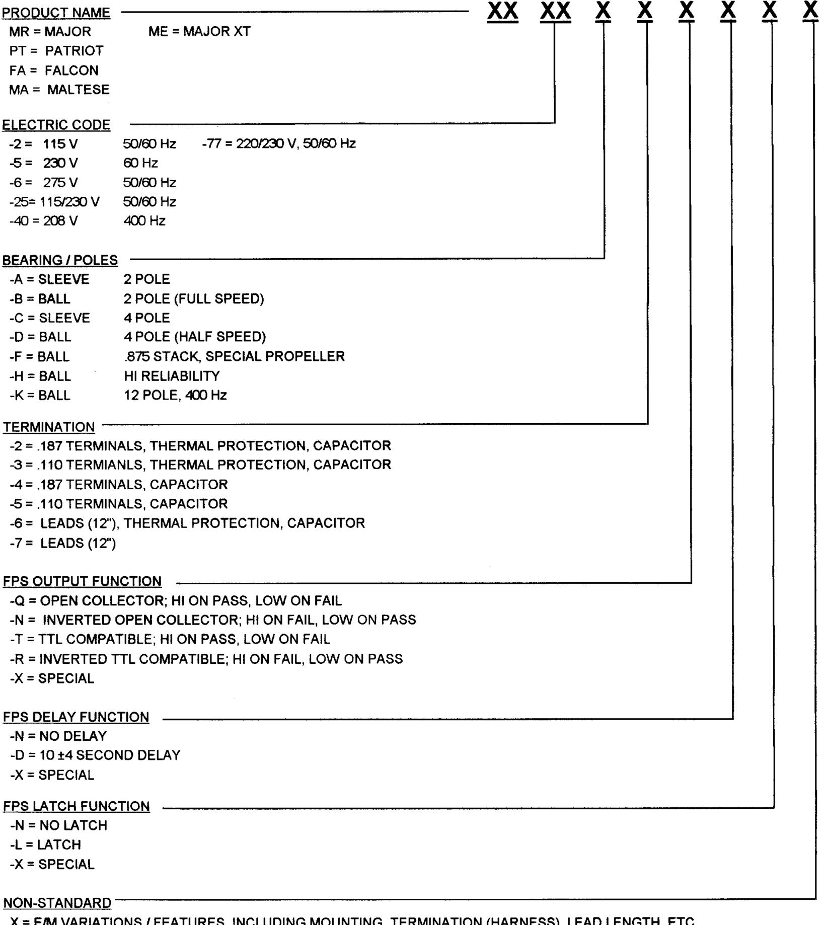
X = E/M VARIATIONS / FEATURES, INCLUDING MOUNTING, TERMINATION (HARNESS), LEAD LENGTH, ETC., NOT AFFECTING BASIC FAN PERFORMANCE.
