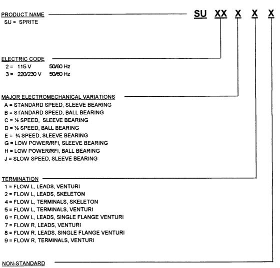
X = E/M VARIATIONS / FEATURES, INCLUDING MOUNTING, TERMINATION (HARNESS), LEAD LENGTH, ETC., NOT AFFECTING BASIC FAN PERFORMANCE.
