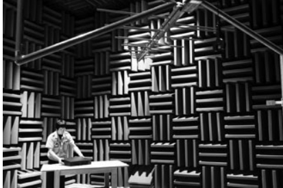
Acoustic radio wave anechoic chamber
