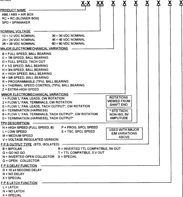
X = MINOR E/M VARIATIONS, LEAD LENGTH, MOUNTING, ETC., NOT AFFECTING BASIC FAN PERFORMANCE. E = ENVIROMENTAL PROTECTION (PER UL SECTION GENERAL)
